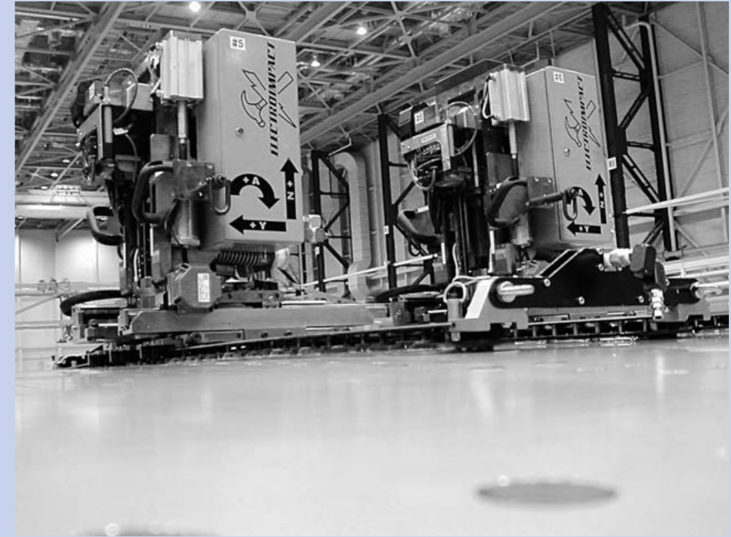
Welding machine for airplane body panels
